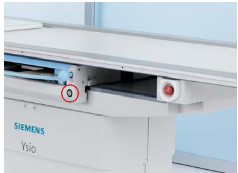
Centering button* Push this "magic button" on the table, and the tube is automatically centered to the table detector for the next examination
