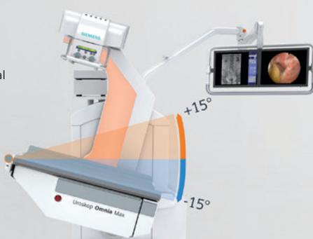
Through a combination of table and tube/detector movements, longitudinal patient coverage can be expanded to up to 98 cm.
